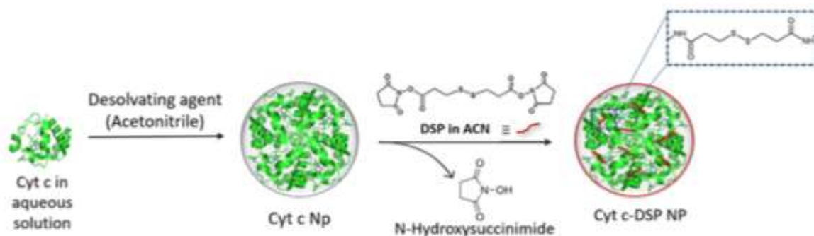
Figure 3.6. Synthesis route of cross-linked Cyt c NP by two-step nanoprecipitation.
