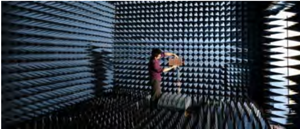
Figure 4 An Anechoic chamber inside the University of Bristol's faculty of engineering photo taken from https://www.bristol.ac.uk/engineering/research/smart/our-labs/anechoic-chamber/ .
