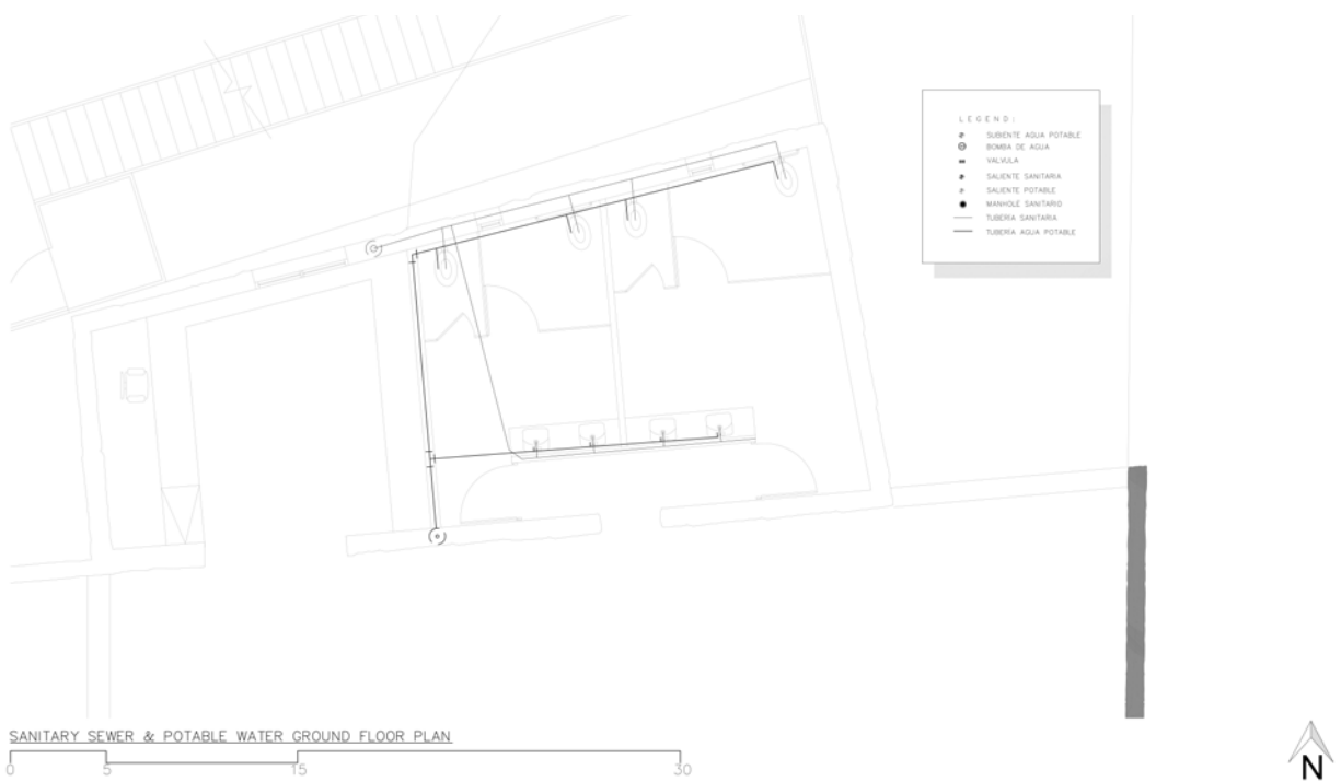
Figure 48. Sanitary Sewer & Potable Water Ground Floor Plan. Diagram by student Reinaldo E. Hernandez Aracena.
