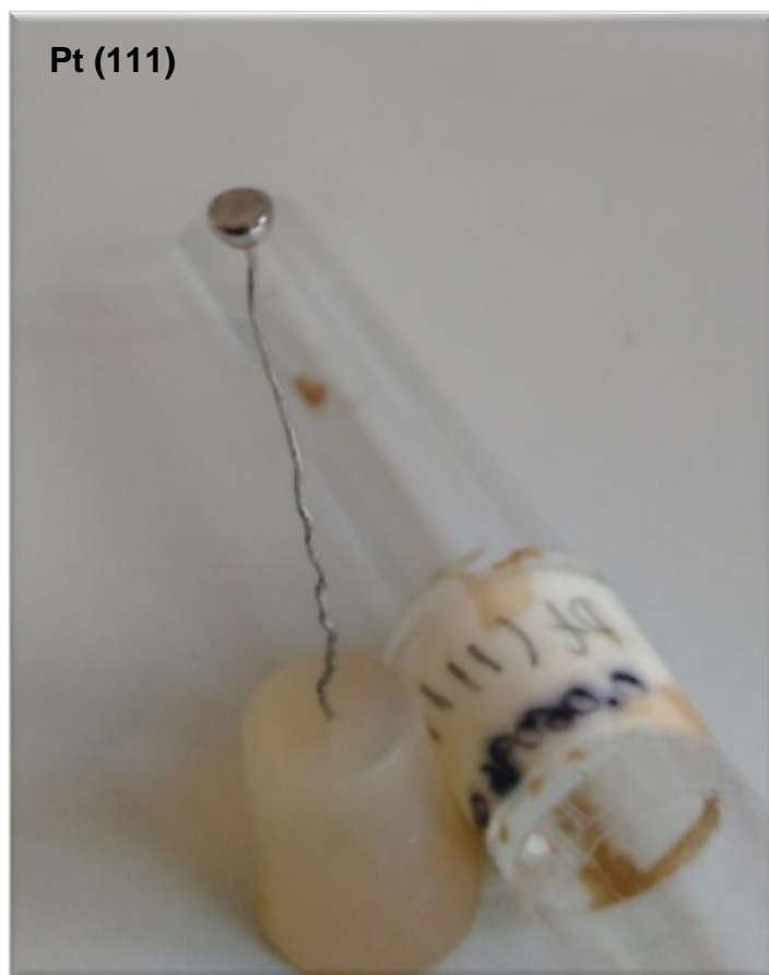
Figure 3-12. Image of Pt (111) single crystal electrode as a reference model for the electrodes used in this research thesis.
