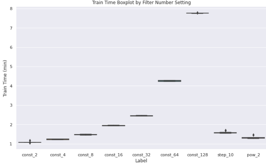
Figure 4.4: AudioMNIST train time for models using the following number of filter sequences: a constant number of filters (const_2, const_4, const_8, const_16, const_32, const_64, const_128); a sequence increasing by increments of 10, step_10 ( [5, 15, 25, 35, 45, 55, 65] ); and a sequence increasing by powers of 2, pow_2 ( [2, 4, 8, 16, 32, 64, 128] )
