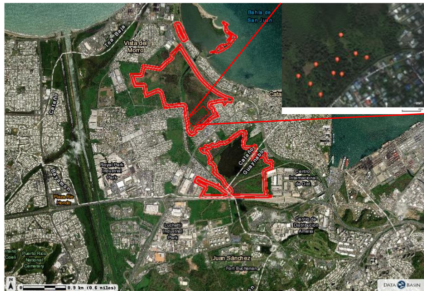
Figure 10 Ciénaga las Cucharillas natural reserve delimitation and location of long-term monitoring wells (red dots)
