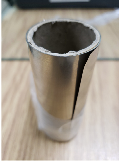
Figure 2.12: Nickel laminate of 0.05 mm thick.
